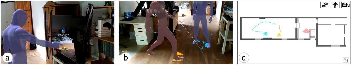
**Figure 6:** (a) Visualization of interactions with the environment, here showing touches on an interactive display with the center one being highlighted. (b) Visualization of where the feet of two avatars are touching the floor of the environment. (c) Floorplan view on the tablet, showing an overview of the environment, the current position and orientation of the analyst, as well as trajectories and the current position of the avatars.
